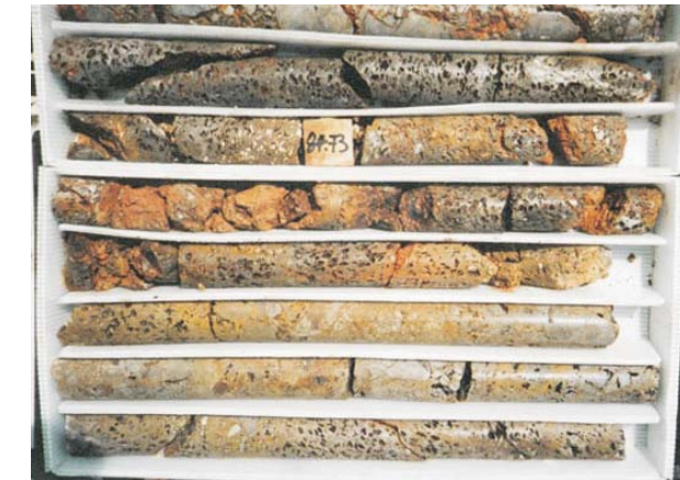
Image: Drill Core from CB05-03 showing intense alteration and vuggy silica.
